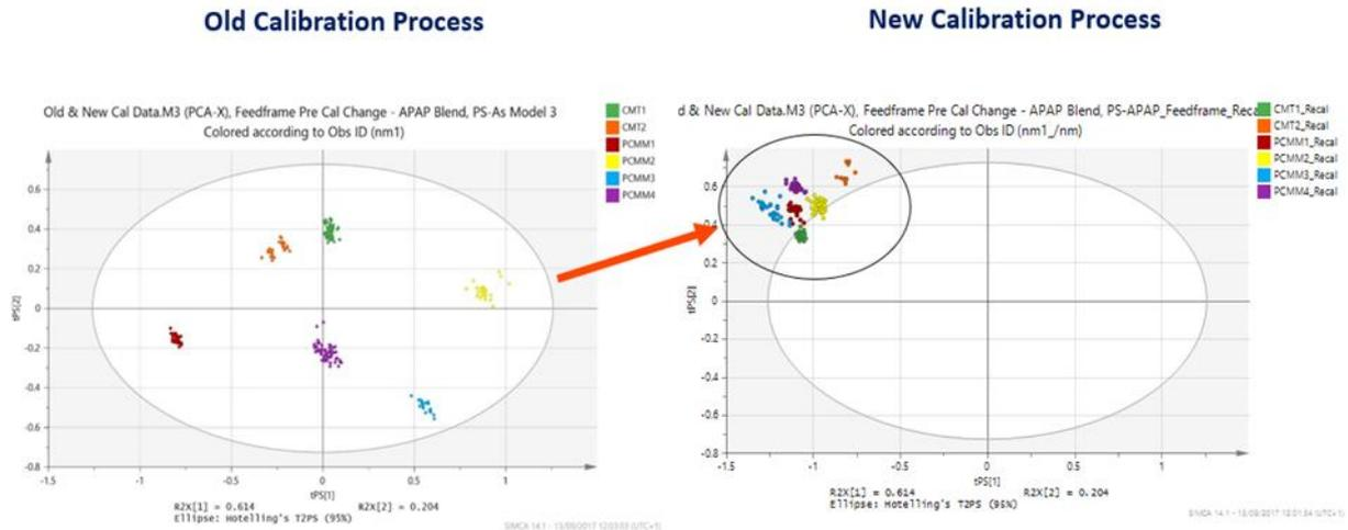
Figure 8. Investigating instrument similarity, with x-axis calibration change
