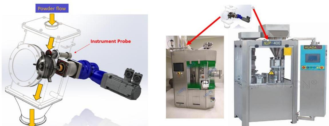
Figure 4. The pharmaceutical application spider wheel. In-let to machines
