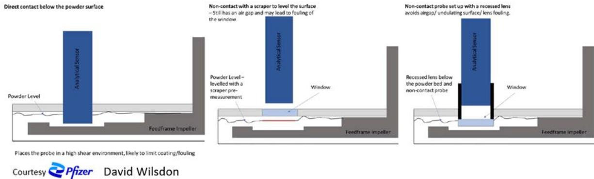
Figure 6. Research into optimum interfacing of a Raman probe
