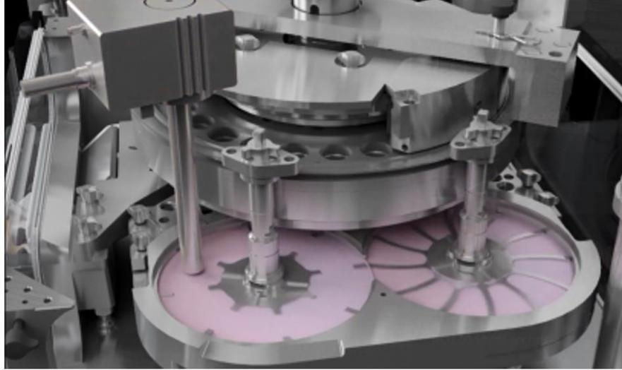
**The insertion of a fiber optic probe into a feedframe**
