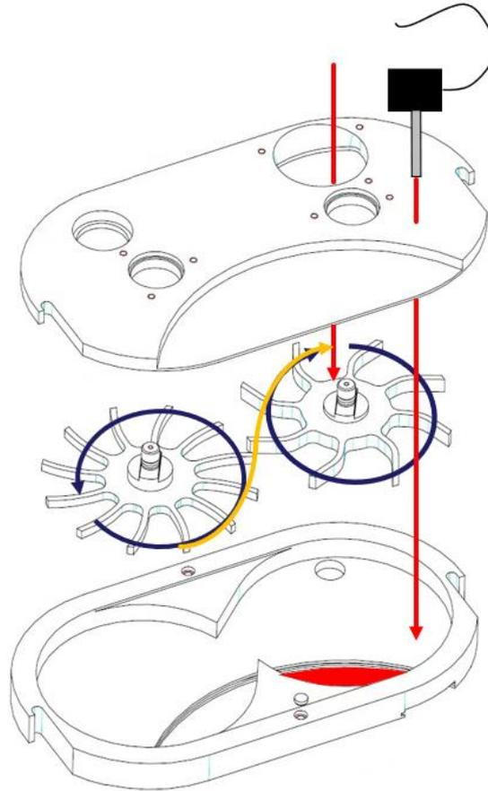
**The direction of powder flow and the position of the probe in the feedframe**
