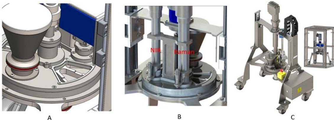
Figure 5A. Simulator internals, 5B. NIR and Raman probes, 5C Rig and enclosure
