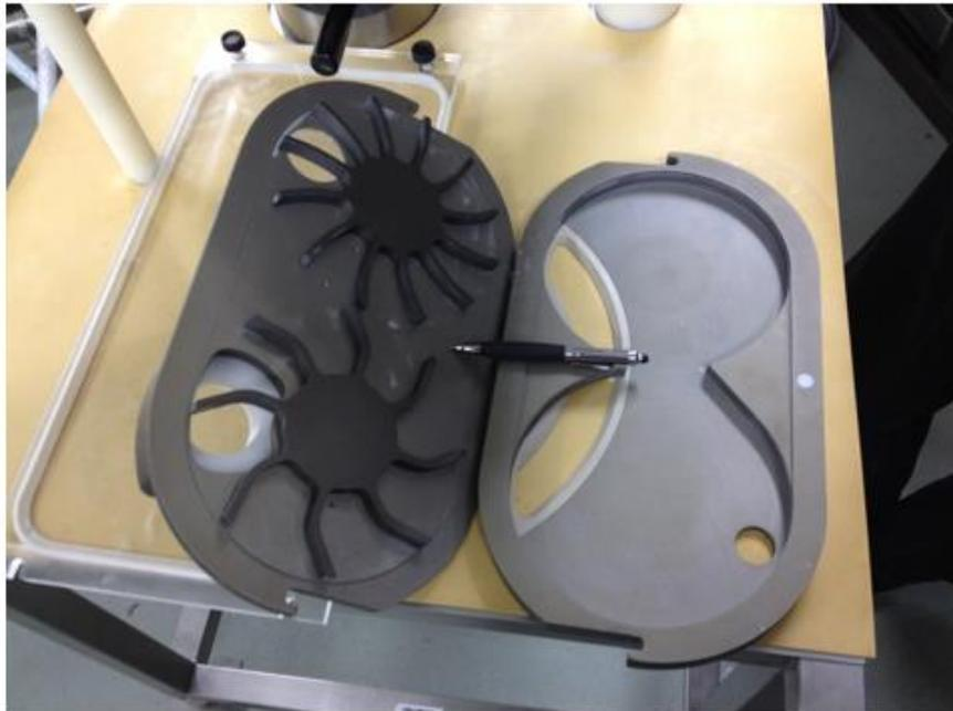
**The internal structure of a tablet press feedframe**
