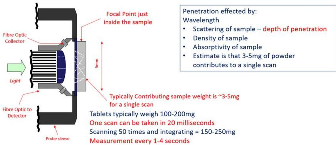
Figure 2. Sampling characteristics of a fiber optic probe
