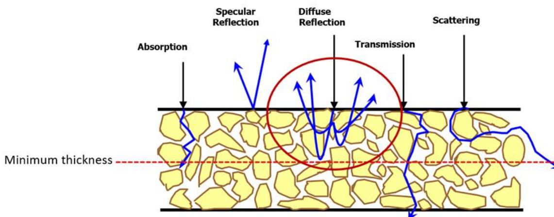
Figure 1. Diffuse reflection and the minimum thickness requirement.
