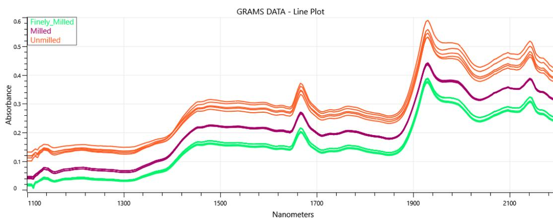
Fig. 6: NIR response for unmilled, milled, and finely milled granules.
