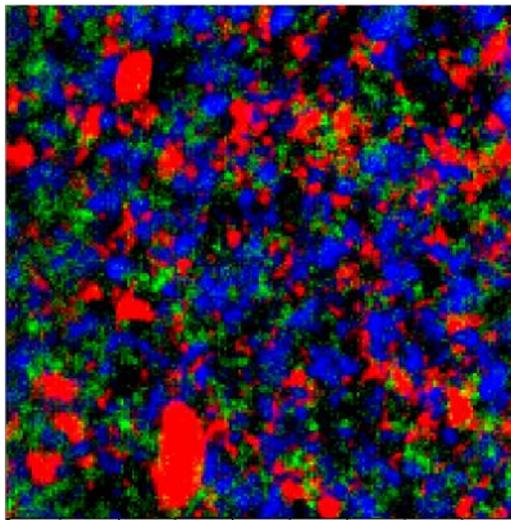
Figure 8: Typical formulation matrix. Red API, Green Lactose, Blue Cellulose.
