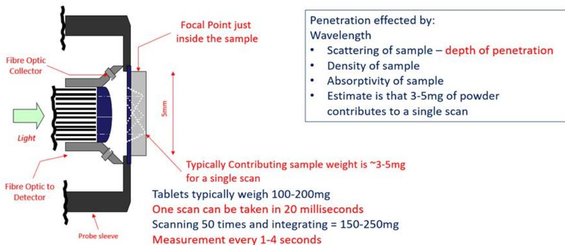
Figure 7: Sampling volume and mass for a diffuse reflectance probe.
